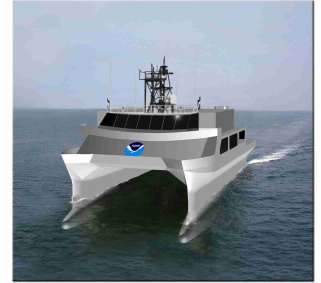
Proposed NOAA SWATH CMV - 29m LOA; 15kt.
