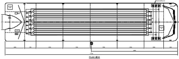
**Fig. 5: Plan View of Z-Pack on A-T-Barge**
