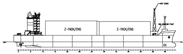
**Fig. 7: Profile of CNGC for Z-Pack Transport**
