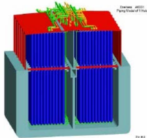
Fig. 3: CNGC Hold Arrangement
