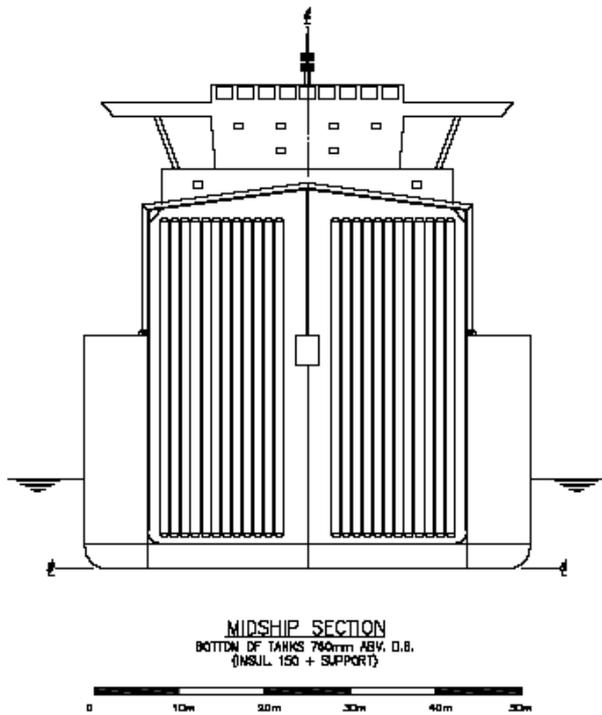
Fig. 1: “V-ship” CNGC Cross-section
