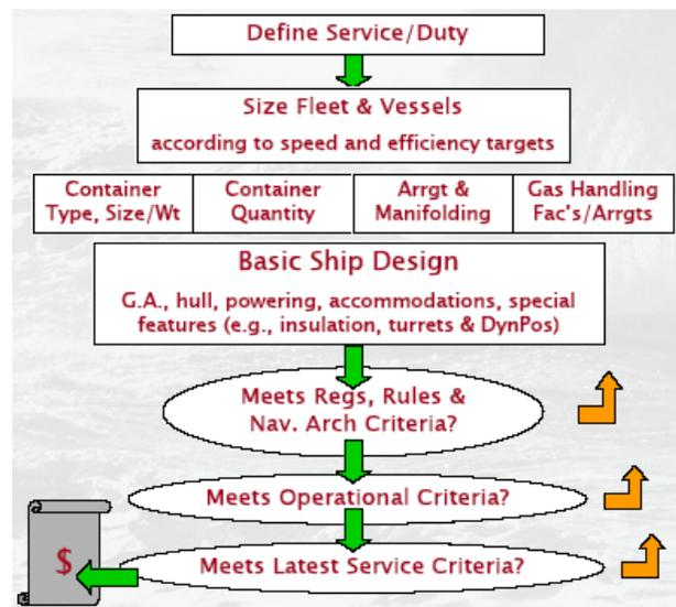
Fig. 2: CNGC Design Flow Process
