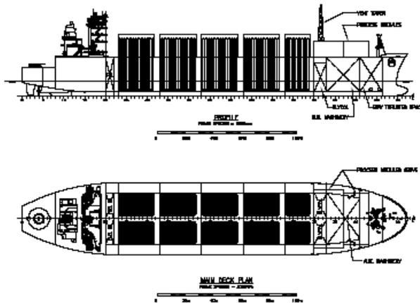
Fig. 4: "V-ship" CNGC example
